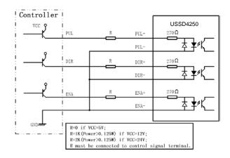
To prevent disruptive noise in the PUL/DIR inputs they should not be bundled together with the motor lead wires. Use twisted part shielded cable and keep separated from motor lines by at least 10 cm.
